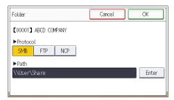
If the network does not allow automatic obtaining of IP addresses, include the destination computer's IP address in the path. For example: if the IP address of the destination computer is "192.168.0.191", and the folder name is "Share", the path will be \\192.168.0.191\Share.
